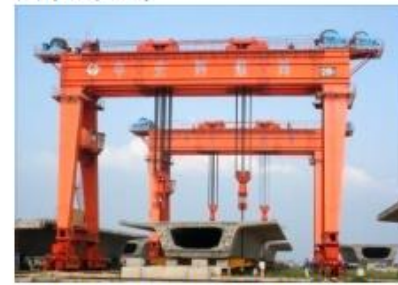
Bridge girder erection machine 架桥机
